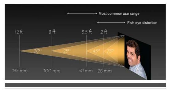
Figure 11: The angle of view varies with lens length (the shorter the lens, the wider the angle of view).
