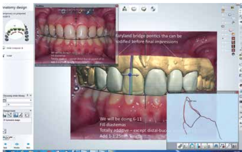
Figure 2: By identifying common landmarks on the photo and the scanned model, the 3D model is synchronized to the 2D digitally overlaid photo using software (3Shape Dental Designer; Copenhagen, Denmark). This allows the laboratory technician to design the outline form created by the dentist as shown in Figure 1. This interconnection of 2D digital design to 3D CAD software improves communication between restorative team members.
